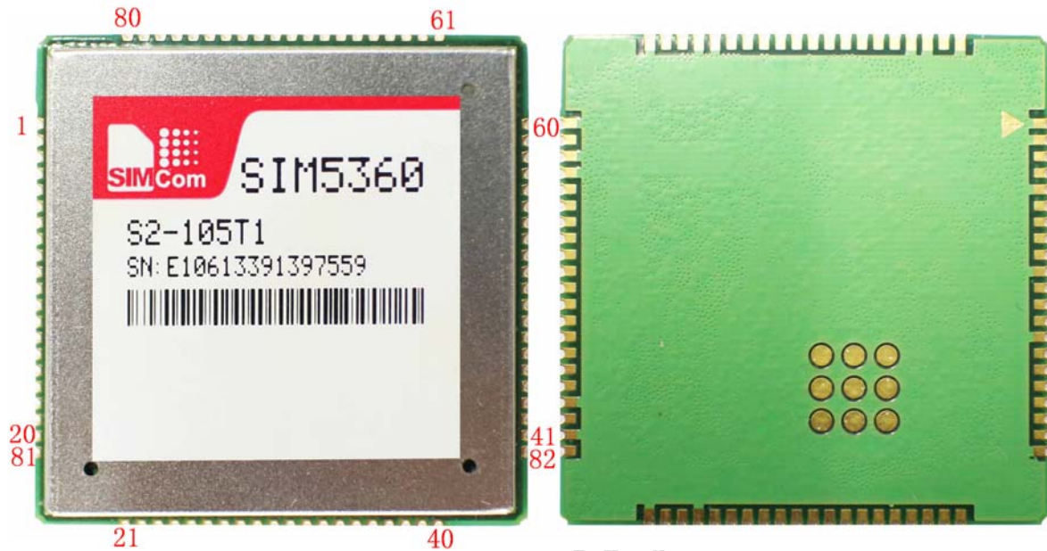
Figure 41: Top and bottom view of SIM5360
